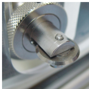
Heavy-Duty roller type harden steel cutter.
